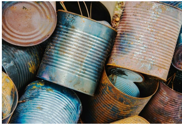
Rust and corrosion on cans can indicate poor storage and a risk of leakage.
