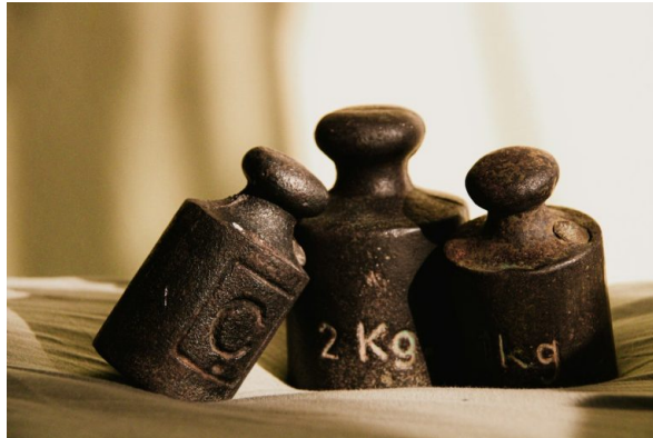
Certified, traceable test weights are used to check the accuracy of scales.
